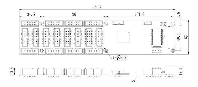
Tolerance: 0.3 Unit: mm
