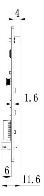
Tolerance: 0.3 Unit: mm
