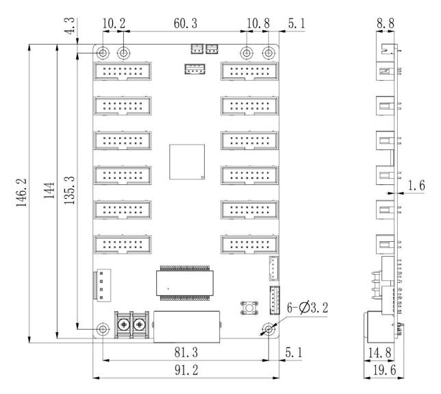
Tolerance: 0.3 Unit: mm
