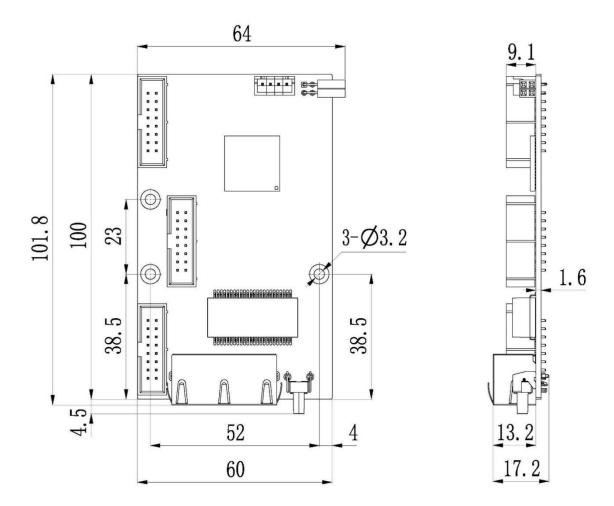
Tolerance: 0.3 Unit: mm
