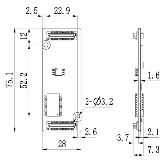
Tolerance: 0.3 Unit: mm
