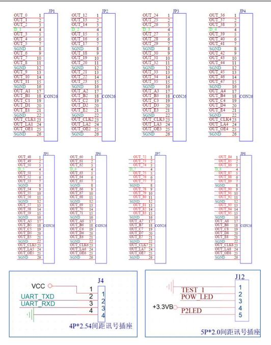
Serial port interface.....external indicator light, button interface
