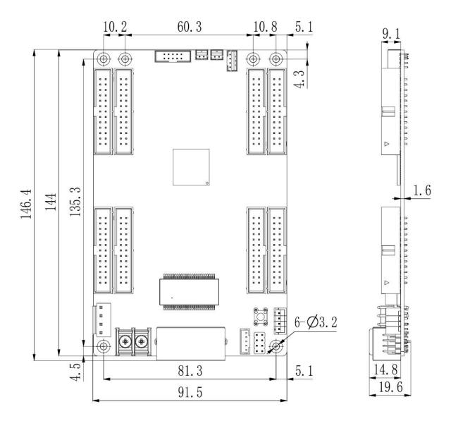
Tolerance: 0.3 Unit: mm
