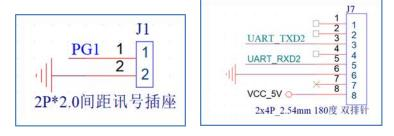
Power detection interface.....external LCD interface
