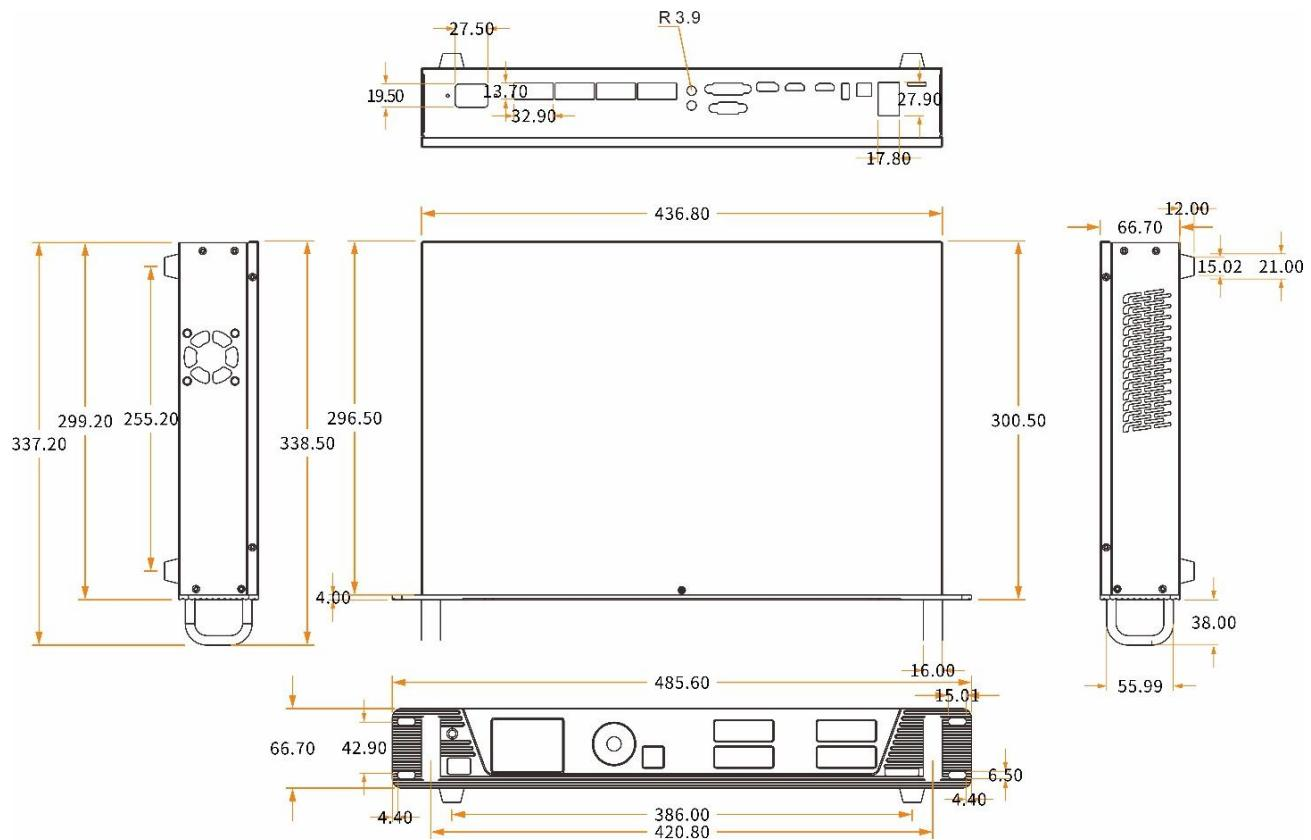
Tolerance:  $\pm 0.3$       Unit: mm
