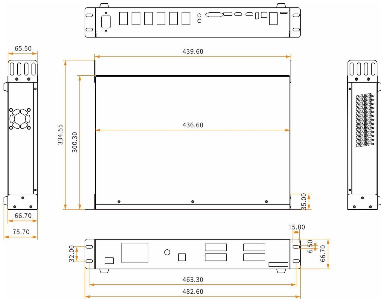
Tolerance: ±0.3    Unit: mm
